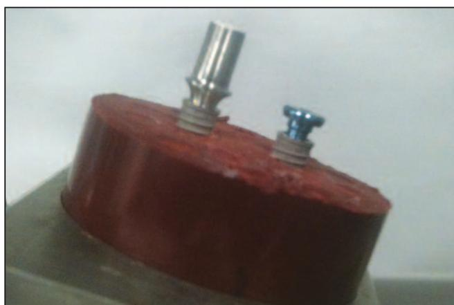
**Figure 2:** Representative implant mounted with 3.0mm simulated resorption.
